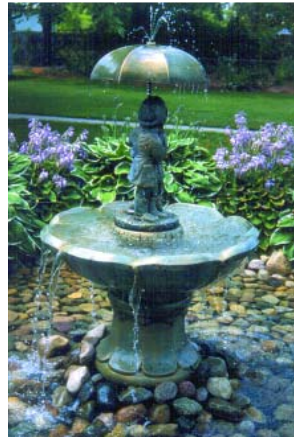
A stand-alone fountain display is run by a concealed reservoir system constructed below the cobbles at the base of the statue.
